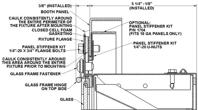
NOTE: LIGHT FIXTURE GLASS FRAME EXTENDS 3/8" INTO BOOTH WHEN MOUNTIED IN BOOTH PANEL
