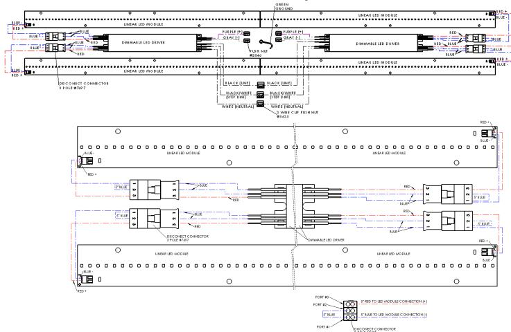
NOTE: THE LED DRIVER IN THIS FIXTURE IS DESIGNED TO OPERATE ON GROUNDED NEUTRAL SYSTEMS ONLY.
