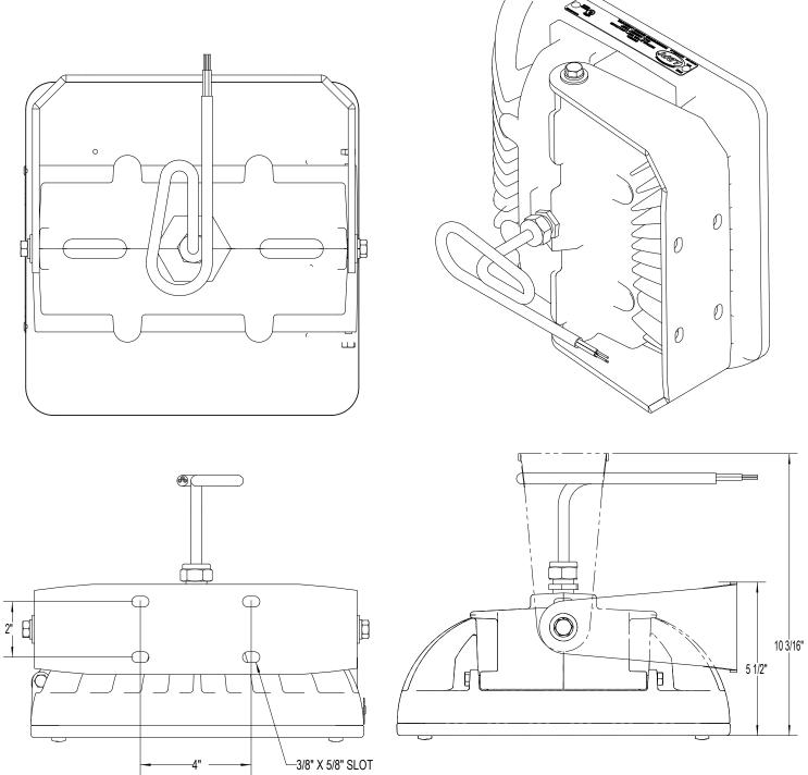
**NOTE:** It is not necessary to remove the yoke mount to install the fixture. If removal of the yoke mount is required, remove the lock nut from each side of the yoke and flex the yoke bracket off of the Set Screw/Studs.
