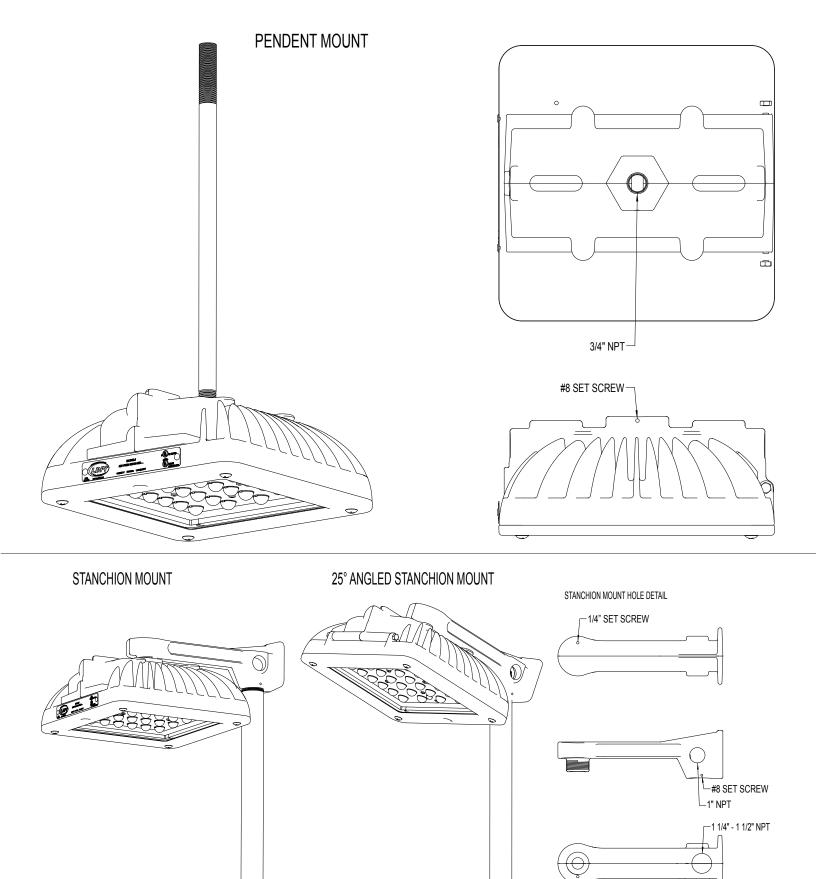
Securely tighten set screws when desired fixture orientation is achieved and the conduit connection is tight.
