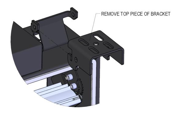
STEP 4: INSTALL TOP BRACKETS TO EXISTING STRUCTURE USING BOLTS.
