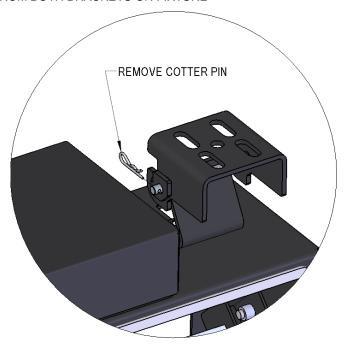
STEP 2: REMOVE CLEVIS PIN FROM BOTH BRACKETS. TOP PIECE OF BRACKET WILL NO BE LOOSE.
